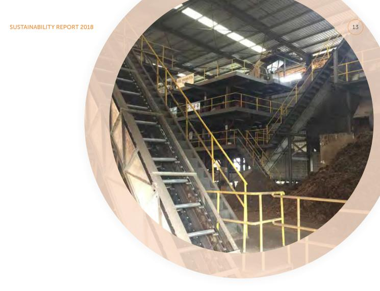
In Mewah Datu Sdn Bhd, we utilize the fiber from empty fruit bunch (EFB) and palm kernel shell (PKS) as boiler fuel to replace fossil fuel. The EFB and PKS are the solid waste from oil palm obtained from milling process. This agricultural waste is considered to have zero life-cycle greenhouse gas emissions up to the point of collection.
